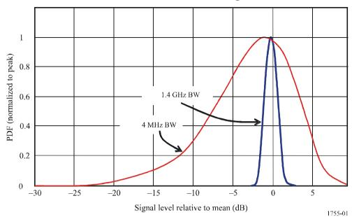
During propagation a sub-nanosecond pulse is dispersed, which may result in Rayleigh fading in the frequency domain. However, each of these reflections is an independent signal so a RAKE receiver can then be used to coherently add the energy in each of the pulses that are received from each of the multipath components to provide a gain over single path reception.
